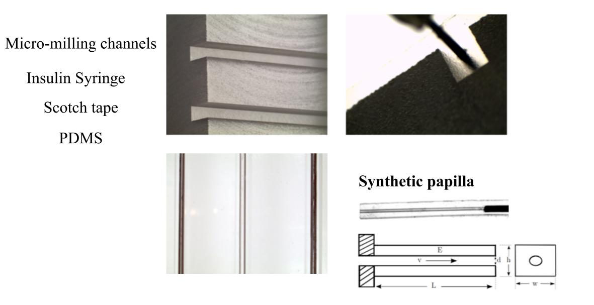
d = 0.81 mm w = 1.60 mm L = 9.5 mm E = 288 kPa h = 1.42 mmThere is no roughness along the inner part of the duct, or an external accordion like geometry
